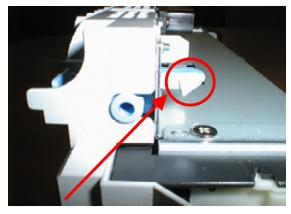
Cracked fuser latch
